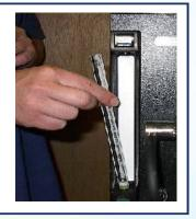
Using needle nose pliers, pull the plastic inserts from each end of the tube being careful not to drop the ball.
