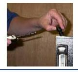
4 Remove the glass tube from the flow meter.
