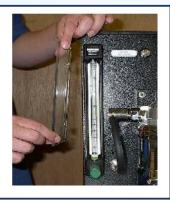
3 Using an allen wrench, remove the plug in the top of the flow meter.
