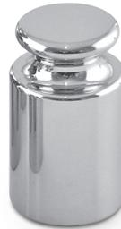
Certified calibration weights are ideal weights to use for scale calibration. They ensure your scale is calibrated properly and ready for the requirements of weighing in the veterinary clinic settings. Consumer weights such as barbells or similar items will not provide an accurate weight to check or calibrate your scale. Using a certified calibration weight will ensure your scale is calibrated correctly and presents accurate weighments for proper animal care.
